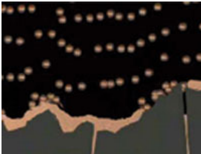
Pic. 2. Particles become structure part of basic metal, they decrease metal surface fatigue, restore microflaws, filling in cracks and burrages
